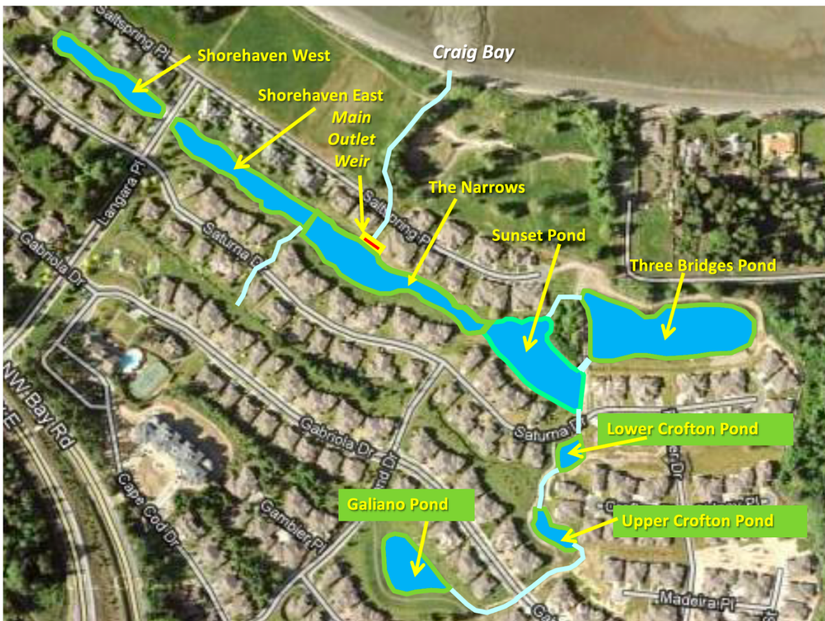
Fig. 1: Craig Bay Estates Pond Stormwater Management System main infrastructure.
